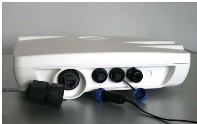
Oberon 350 - External IP 65 connectors & I/O
