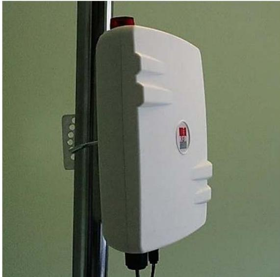
RFID UHF Mid Range Antenna with integrated Reader, Industrial Series, RedWave Smart FlyBoard with CPU & I/O
