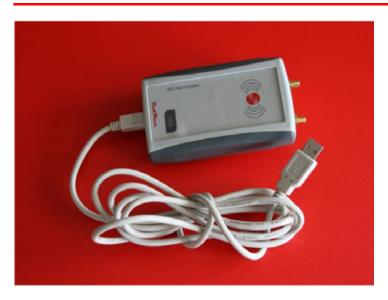
RedWave Short Range Controller UHF EPC USB in case with 2 external multiplexed antenna.
