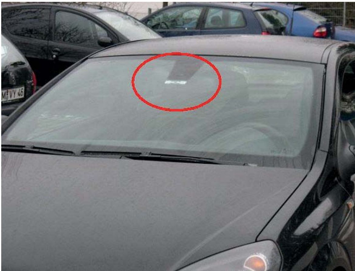
Figure 11: Mounting of the transponder
