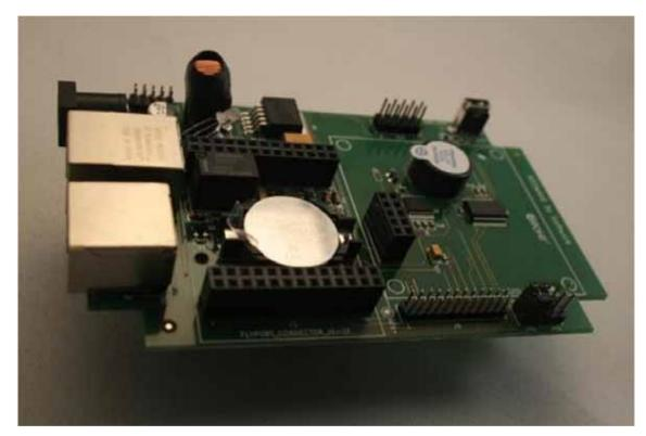
OEM Developer Smart Board (Lan, WiFi, GSM/GPRS) for RFID OBID Controller HF & UHF with CPU processor & I/O. Compatible with
