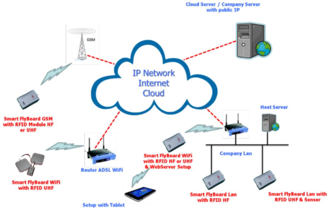
All RFID Device based on the **RFID RedWave Smart FlyBoard** are available in 3 versions (Lan, WiFi, GSM/GPRS), specifically projected and produced for RFID OBID Controller HF & UHF of FEIG Electronic. The RFID RedWave Smart FlyBoard is equipped with CPU processor & I/O, so that it helps to create flexible RFID architecture, operating in both frequencies (HF and UHF), building them like “LEGO bricks” according to the specific needs of the RFID project.
